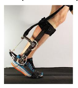
The Stanford Biomechatronics Lab invites you to participate in research that focuses on improving controllers for robotic exoskeletons (assistive devices at the ankle). The development of novel exoskeleton control aims to decrease the effort of walking by providing assistance to the sound
